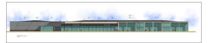
The design of the buildings involves extensive glazing to the frontages, with additional glazing on the Cartwright Lane side of the food and drink 'pod'. These are to be clad in a mix of blue brick, stone rainscreen cladding (buff) and grey ceramic tile. The rear elevations (north and east facing) are microrib composite cladding panels laid vertically and randomly of different shades of green and buff to break up these extensive elevations.
